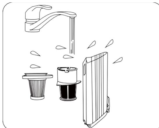
Wash the dust cup and both filters thoroughly with water.
